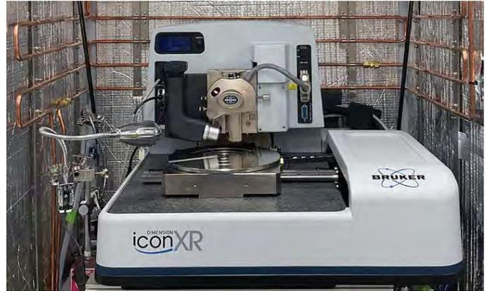
Bruker AFM for Amplitude-Modulation imaging (AM-AFM)
